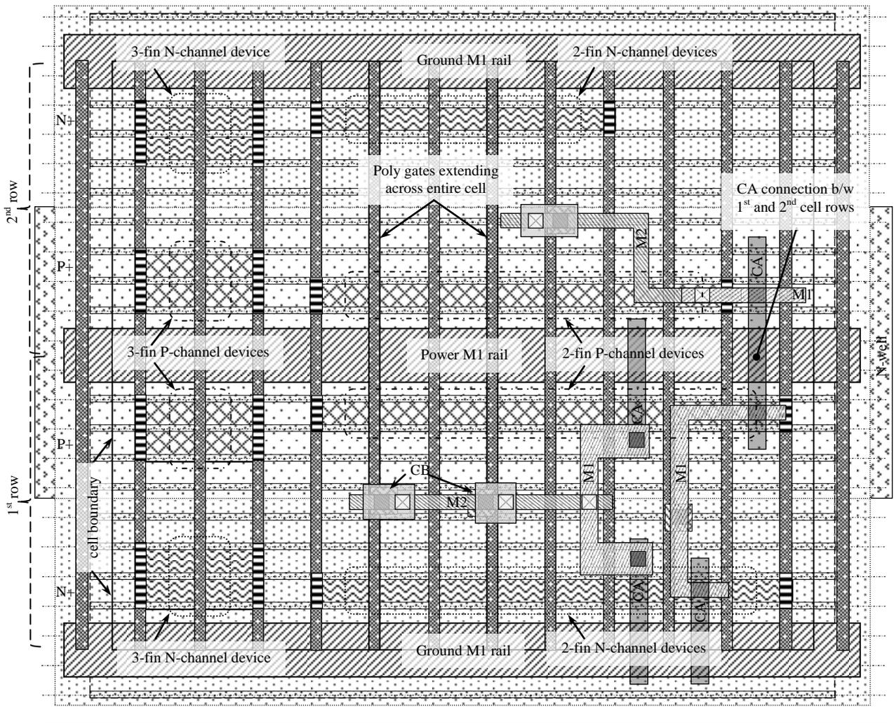
**Fig. 6. Generalized structure of double-height cell layout**
