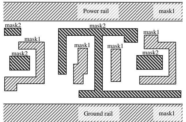
Fig. 4. Coloring of metal routing due to BEOL double patterning
