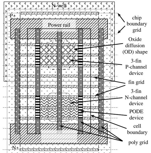
Fig. 2. Simplified layout template of standard cell in FinFET technology
