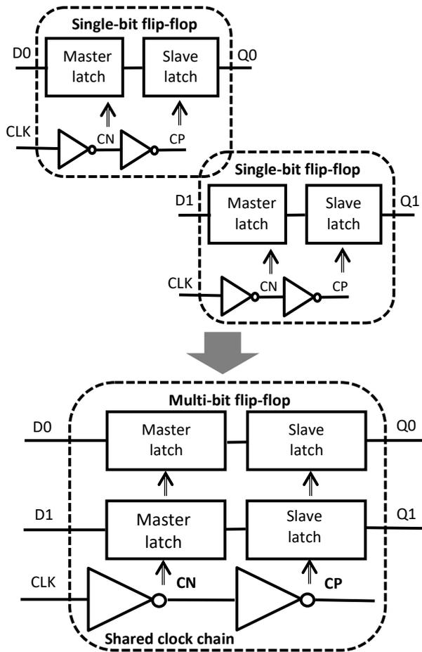
Fig. 7. General circuit architecture of multi-bit flip-flop
