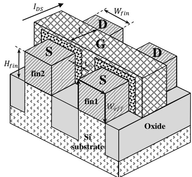
**Fig. 1.** 2-fins FinFET device structure with geometric parameters
