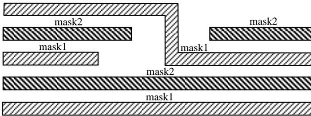
Fig. 5. Example of routing limitation due to DPT
